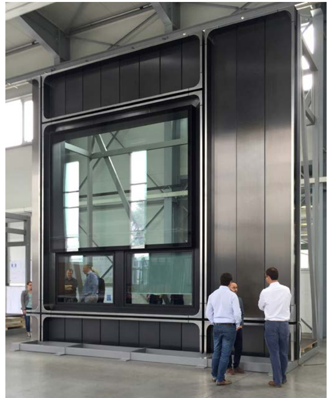
Office cladding visual mock-up
