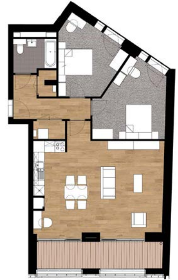
Plan of a typical two-bedroom apartment, with the winter garden leading off the main living space.
